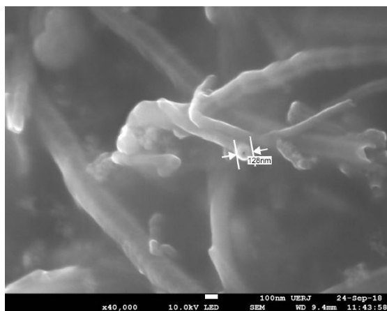
Figure 3: Carbon nanotubes in the sample of PLA graphene
